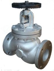
**Bolted Bonnet** is the most common design because there is practically no limitation on size. <u>Multiple bolting</u> permits equalized sealing pressure on the gasket against high pressure encountered in iron globe and angle valve applications.
