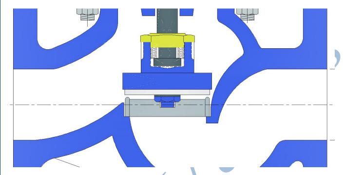
Body Test Pressure: 60 Kg/cm<sup>2</sup>. Seat Test Pressure: 40 Kg/cm<sup>2</sup>
