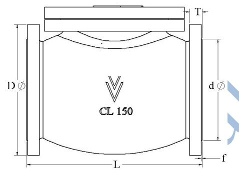
Body Test Pressure: 425 psig Hyd. Seat Test Pressure: 300 psig Hyd.
